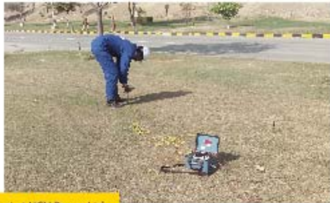
Soil Resistivity measurement at UCH Power Ltd
