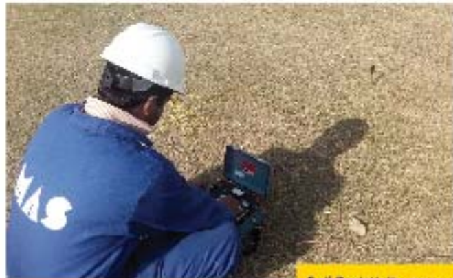
Soil Resistivity measurement at UCH Power Ltd
