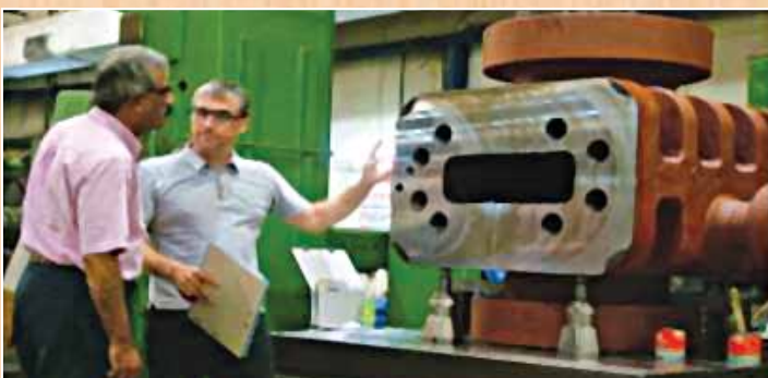
OGDCL Inspector, Mr. Tuaha Jamil inspecting BOP while it was under repair at WESCO A.D. workshop
